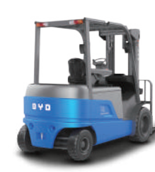
ECB35 Load capacity: 3.5 ton Curb weight: 5,440 kg Min. turning radius: 2,210 mm Voltage: 80 V Battery capacity: 540 Ah
