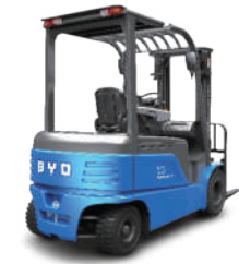
ECB30 Load capacity: 3.0 ton Curb weight: 4,840 kg Min. turning radius: 2,210 mm Voltage: 80 V Battery capacity: 270Ah/540Ah
